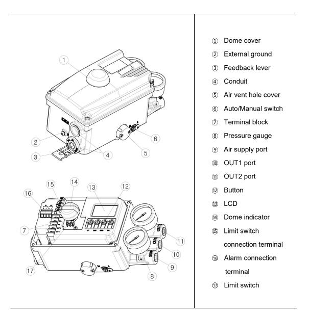
Note: Only Limit switch type product is equipped with Dome indicator.
